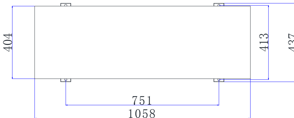
Figure 2- 15 Mounting base shape and size of DKFXF(C) -014SCI, 017SCII, 018SCI Unit(mm)
